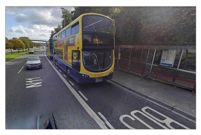
Figure 7.2 Where space permits double bus bay should be provided where more than one bus is expected to arrive at a bus stop simultaneously (source: Google)
