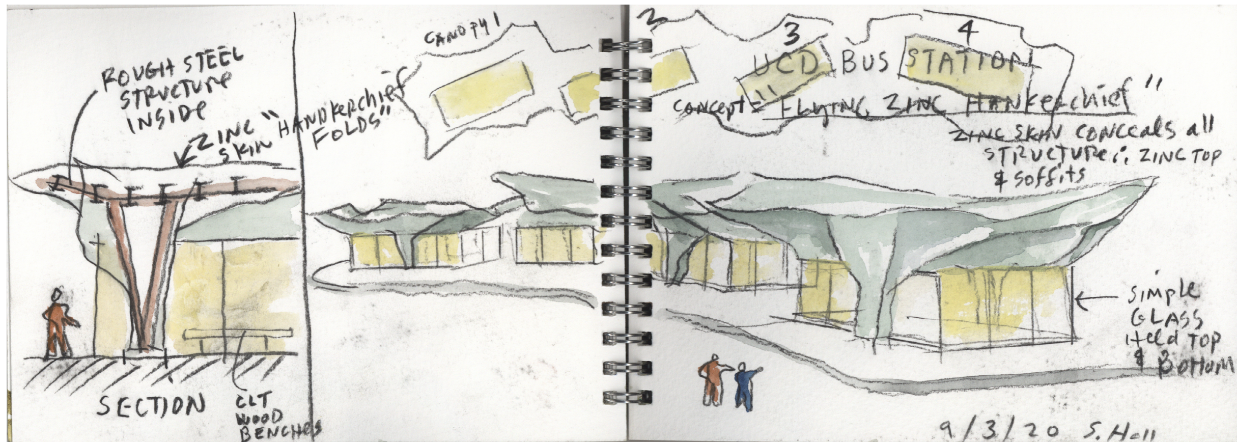
Figure 3.1.3.1 - Zinc clad handkerchief geometry enables surreally floating geometry concealing rational and efficient steel structure
