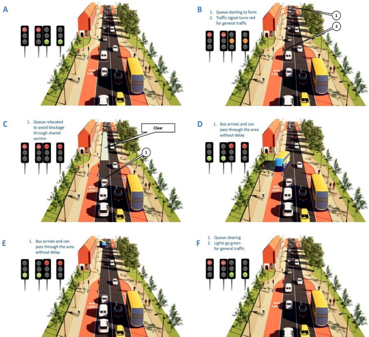
Image 4.15: Signal Controlled Priority (SCP) Schematic Operation (Source: PDGB)
