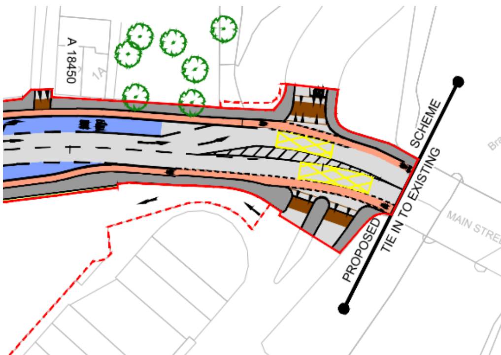
Image 4.19: BusConnects Design tie-in to the Existing
