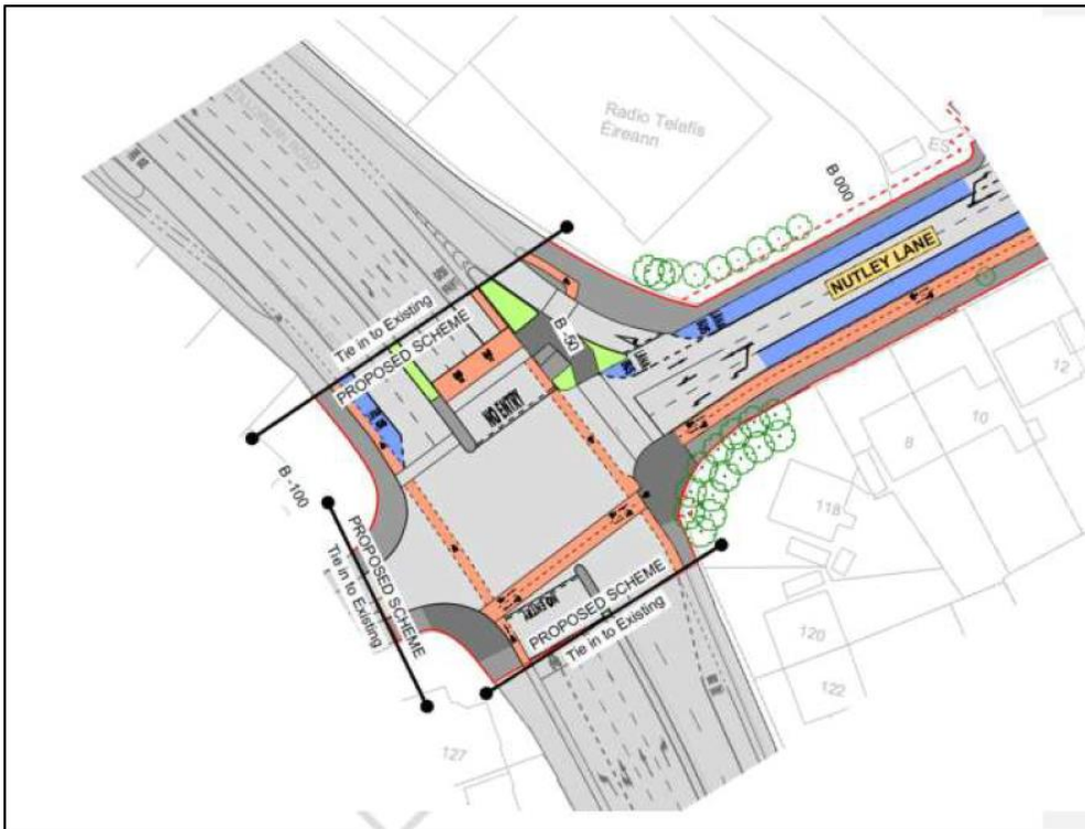
Image 4.22: Preliminary Design of the Belfield / Blackrock to City Centre Core Bus Corridor Scheme at Nutley Lane, Tying into the Existing R138 Stillorgan Road / Nutley Lane Junction Layout
